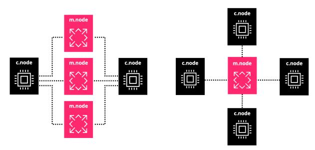
Silk allows you to scale up capacity by adding more m.nodes to your environment's base configuration, without requiring any additional resources. Vertical scaling in Silk provides several cost and performance benefits, including:
