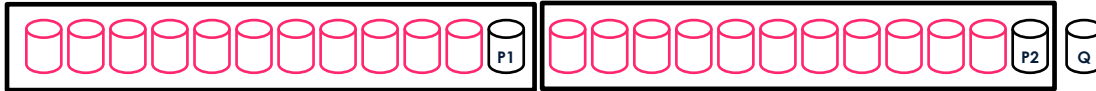
Figure 9: K-RAID logical layout of two RAID groups and a Q parity for both groups
