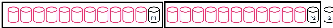
Figure 5: K-RAID logical layout of two RAID groups and a Q parity for both groups
